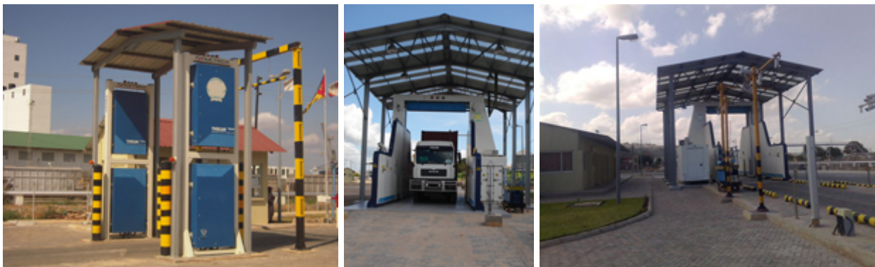
X-Ray Scanner, Fast Scan, 6 MeV, Dual Power System, installed at the port of Nacala (April 2010) and control room operations
