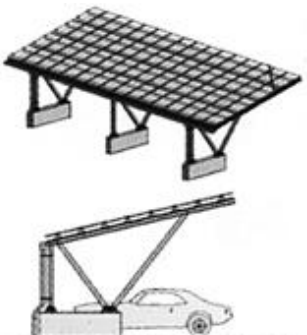
1-row vehicle arrangement (max.depth 6m)
