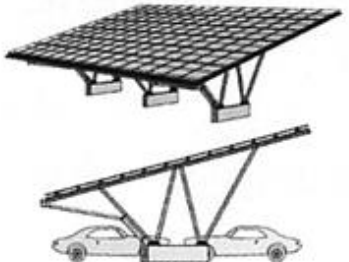
2-row vehicle arrangement ① (max.depth 13.5m)
